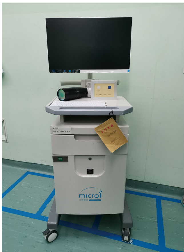
FIGURE 1 Near-infrared fluorescence imaging system mediated by blue dye, which is composed of a computer, a monitor screen, and a hand-held probe for exciting near-infrared light [Color figure can be viewed at wileyonlinelibrary.com ]
